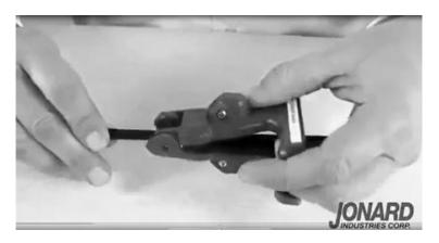
Figure 4 – Position the cable slitter over the cable and close the tool. (Photo courtesy of Jonard Industries, Corp)
