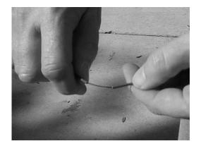
Figure 9 – Flex and snap the buffer tube at the score line.
