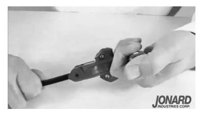
Figure 5 – Pull the cable slitter along the cable to slit the jacket. (Photo courtesy of Jonard Industries, Corp)
